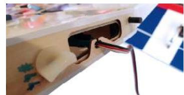
3. Install the elevator servo, rudder servo, wings servo, the rudder servo connected up with the provided push rods and ball links.
