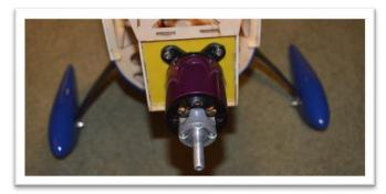
Larger diameter motors like the AJ3910-24p-660KV will require some additional work.
