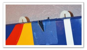
Use 30 minute epoxy to glue the control horns in place. Center the control horn, peal the masking tape away, and clean up with alcohol.
