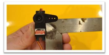
Attach an 18" servo extension onto the elevator servo lead and use a safety clip to secure the connection.
