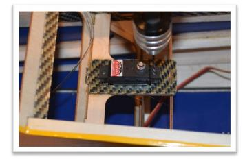
Start the cable assembly at the servo end inside the fuselage. Straighten out the cables and determine which cable is on the left and which cable is on the right. The cables should cross inside the fuselage once. The cable on the left at the rudder should be connected to the servo control horn on the right.
