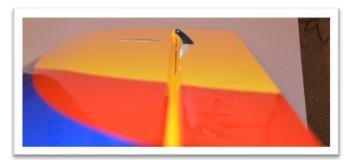
Allow the epoxy to partially cure. Peel away the masking tape after the epoxy is securely holding the control horn in place and still soft enough to easily remove the tape. Set the wing aside and let the epoxy fully cure.
