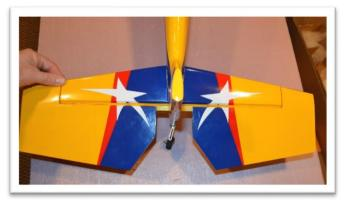
Apply masking tape around the jointer slot in the right elevator half.
