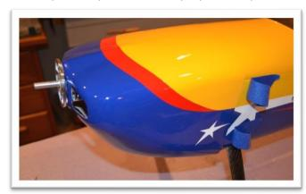
Drill a 1/16" hole through the cowl and the fuselage at the marks you made.
