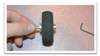
Insert the wheel and axel into the wheel pant, then into landing gear. Align the wheel pant indentation with the landing gear. Add a nylon lock nut and tighten.
