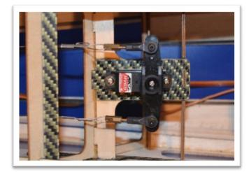
Thread on 2 crush sleeves and the brass cable eye.
