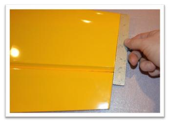
Apply a piece of tape next to each hinge. This will help you locate the hinges when you begin gluing them. Check the aileron position at the hinges and wing tip again before gluing.
