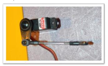
Check the length of the assembly to the servo arm with the aileron level with the wing. When the correct length of the assembly is found, connect the ball link to the servo arm. (Always adjust the connecting rod length with the servo powered up and centered.)
