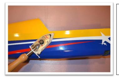
At 200-220°F (93-104°C) the adhesive on UltraCote® becomes active allowing the covering to be attached to the model. While 220° will fully bond the covering to the model it is well below the temperature that causes UltraCote® to shrink.
