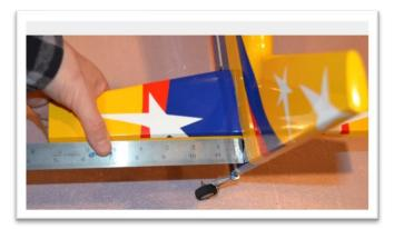
Install and center the main wing tube. Look at the plane from the back forward to make sure that the horizontal stabilizer is parallel with the wing tube. Notice that the horizontal stabilizer is tapered which may obscure the actual alignment. If the stabilizer is not aligned use shims or sand inside the pocket until it's parallel.
