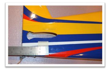
Slid the horizontal stabilizer through the fuselage pushing it all the way forward. Center it side to side using a ruler or tape measure.
