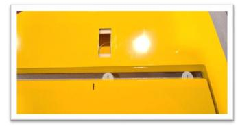
The hinges should already be glued into the ailerons. Give each of them a little pull to ensure they are securely attached. It's better to find a loose hinge now rather than during a flight.
