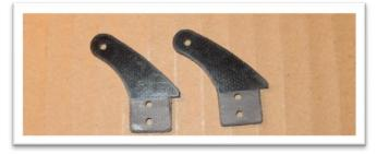
Test fit the control horn in the slot. Trim or file the slot as needed to achieve a snug fit. (Be careful you don't poke through the other side of the aileron.)
