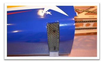
Install the carbon fiber landing gear using 2 washers from the parts bag and the socket head screws. Apply a drop of thread locker as you install these screws.
