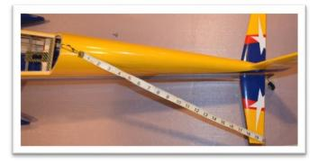
Once the horizontal stabilizer is positioned glue it in place with thin CA glue. Wick glue in on left and right sides, top and bottom. The use of an applicator tip is suggested to control the flow of thin CA glue and get it exactly where you want it.
