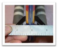
Position the rudder and control horn so gravity does not reposition the control horn as the epoxy cures.
