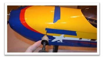
Remove the cowl and thread the screws into the fuselage holes. Remove the screws and add a drop of CA clue to harden the wood around each hole. When the glue is dry reinstall the cowl.
