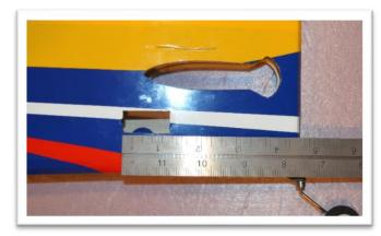
The servo pocket on the <u>right</u> side of the fuselage is used for the rudder servo if you decide to use a push-pull configuration. <u>Do not cut this pocket open if you plan to use the pull-pull cable for the rudder.</u>
