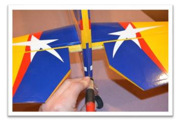
Slip each rudder hinges into a slot. Check the gap at the top of the vertical stabilizer and the rudder counter balance. Push the rudder tight against the stabilizer closing the gap between the two of them. Move the rudder to its maximum desired deflection. Experiment with the hinge position finding the best fit before gluing.
