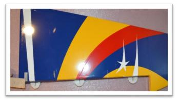
Cut the covering to expose the lower control horn slot on the right side of the rudder.
