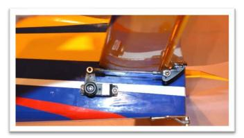
Adjust the length of the connecting rod to the servo arm with the elevator aligned with the stabilizer. When the correct length of the assembly is found, connect the ball link to the elevator control arm on the inside as shown. (Always adjust the connecting rod length with the servo powered up and centered.)
