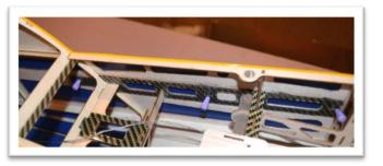
Cut open the pocket just after the second small hole. This is where the aileron servo wire will enter the fuselage.
