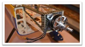
Solder battery and motor connections to your ESC before installing it if needed. Use nylon zip ties or a hook & loop strap to secure the ESC to the bottom of the motor box.
