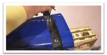
The filler block can be held in position with strips of covering material, packing tape, or it can be held in position with hook and loop material as described below.
