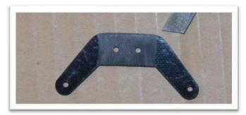
Tests fit the control horn to the slot. Use a file to modify the slot as needed. Center it side to side and align the holes with the hinge line. The control horn should be symmetrical about the hinge line.
