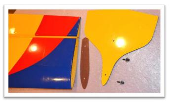
Assemble the spacer plate and the side force generator to the wing with the supplied 3mm screws and washers.
