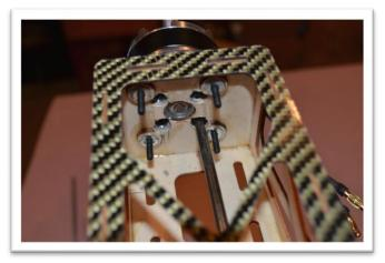
After the test fit be reassemble it with removeable thread locker.
