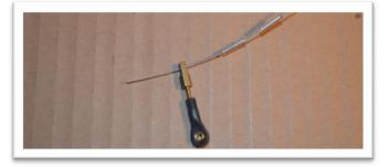
Loop around the cable eye and go back through a crush sleeve.
