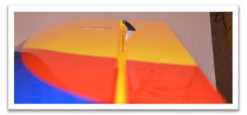
With the control horn in position apply masking tape around it. This will keep excess epoxy off the covering.
