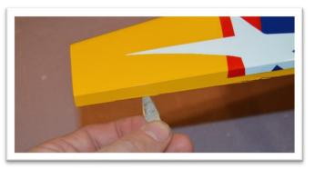
Test fit the elevator joiner plate to the opposite elevator half. Ensure the elevator halves are not twisted. Hold one half of the elevator in position and check the alignment of the other side. Check the gaps at the ends of the stabilizer. Adjust the slot in the elevator or file the edges of the jointer plate as needed to achieve a good fit.
