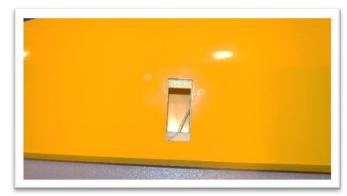
Gently pull off the servo wire installation string and temporarily secure it out of the way. Do not pull it out of the wing. (If there is glue left behind scrape it off so the wood mounting surface is flat.)
