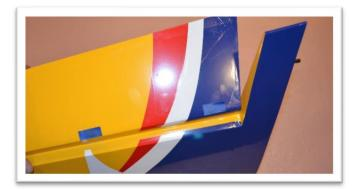
Start with the hinge near the wing tip. Flex the aileron slightly and apply a few drops of thin CA glue to one side. Flex the aileron to its maximum position and return to center. Then glue the opposite side.
