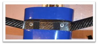
Then cut or sand recesses into the filler block to accommodate the thickness of the hook and loop tape. Start with shallow cuts and test fit it to the landing gear. If the filler block does not sit flush with the bottom of the airplane cut and sand a little more. Continue until you get a nice fit and the hook and loop tape has a firm grasp. It may also be necessary to cut some clearance around the holes for the screws and washers.
