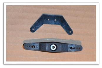
Assemble the ball links to the control arm using the 2mm screws and lock nuts.
