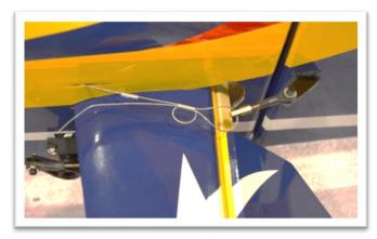
Remove the tape and adjust the cable lengths to center the rudder by turning the cable eyes into the ball links.
