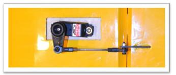
Carefully locate the mounting holes in the side force generators and trim away the covering. The wing tips have a blind nut installed beneath the covering. Use a hobby knife to trim away the covering. (Use the holes in a spacer plate to help locate the holes in the wing tip.)
