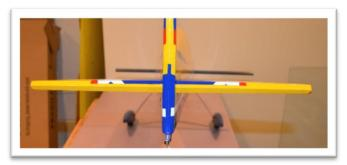
Position the stabilizer perpendicular to the fuselage and parallel to the main wing tube. Measure the distance between the canopy latch and the corners of the horizontal stabilizer. Adjust the stabilizer until the measurements on both sides are equal. Continue checking the stabilizer to ensure it is still centered side to side as described above. Extra time spent here will go a long way to improve the flight characteristics of your airplane.
