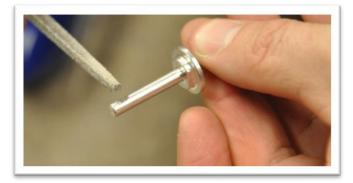
Install a wheel on the axel with a wheel collar. Position the collar set screw over the flat you filed.
