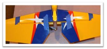
After the epoxy has had plenty of time to cure remove all the masking tape.
