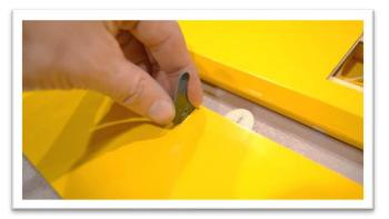
The control horn should go all the way in until the shoulder contacts the aileron. The linkage hole in the control horn should be aligned with the hinge centerline.
