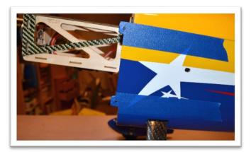
Peel back the tape so you can slide the cowl on. Center it using the spinner backer plate. Leave a .06-.09" (1.5-2mm) space behind the back plate. When you've found the cowl position you like securely tape it into position.
