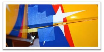
Remove all masking tape right away and clean again. Position the elevator as your did during the test fit. Check it at the ends of the stabilizer.
