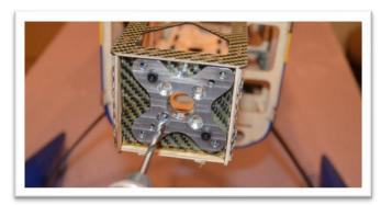
Remove the motor mount and enlarge the holes to 5/16". (A little CA glue and a file will help clean up the carbon fiber strands and hole shape.)
