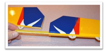
Install a control horn in the elevator using the same procedure used when assembling the ailerons. <u>Make sure you are working with the left elevator half.</u>
