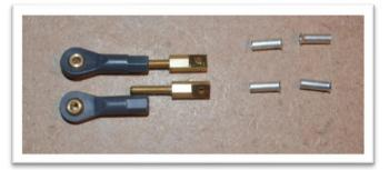
Connect the ball links to the rudder servo arm using a pair of holes that match the rudder control horn holes as close as possible.
