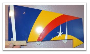
The push-pull control horn is located approximately 9/16" from the bottom of the rudder.
