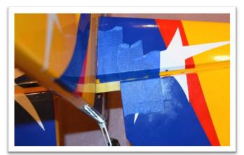
Use a paper towel and alcohol to wipe away excess epoxy that is pushed out. Remember to check the bottom side.
