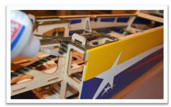
Locate the mounting holes for the wing. Use an iron to seal the covering around the edges of the pocket before trimming. There will be 2 holes for wing alignment pins, 1 hole for the wing bolt, 1 slot for the servo lead, and 1 large hole for the wing tube. Measuring from the front edge of the firewall the holes can be found at 3", 5 7/8", 7 1/4", 12 3/4". You can also locate the holes by pocking a pin through the covering from the inside out.
