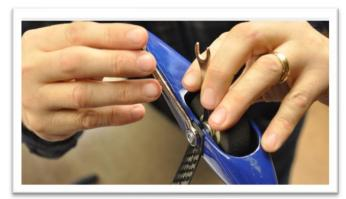
Install the tailwheel using 2 of the 3 wood screws. Position the joint of the tail wheel assembly directly over the rudder hinge line and mark the position of the screws. Turn the screws into the fuselage and rudder. Remove the screws, add a drop of thin CA glue to each hole to strengthen the wood, and reinstall the screws.
