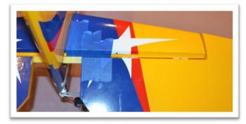
Put the right elevator half in position on the horizontal stabilizer.
