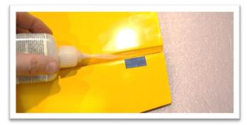
Close the gap between the aileron and wing to the desired position at the fuselage end of the wing half. Flex the aileron slightly and apply a few drops of thin CA glue to both sides of the hinge. Again move the aileron back and forth to its maximum positions. Once the end hinges are securely positioned you can apply a few drops of thin CA to both sides of the remaining hinges.
