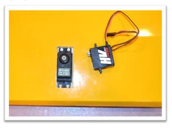
Fit the adapter plate into the servo pocket if you are using the micro size servo. You may need to sand the edges slightly to fit it in. The front corner of the servo pocket should be tilted away from the aileron control horn as shown.
