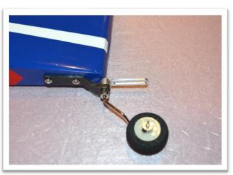
The third screw is used to secure the tiller arm to the rudder after it's installed. Do not fully tighten the tiller arm screw. The slot in the tiller arm allows the rudder to move freely.
