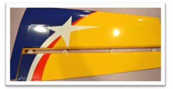
The wings are already slotted for the hinges. Use a covering iron to secure the covering along the edge of the wings. Look at the wing hinge slots closely. Make sure the covering will not interfere when gluing the hinges. Cut away any covering that covers the hinge slot.
