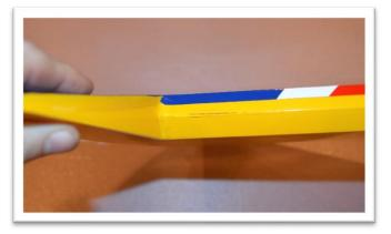
Slip each of the aileron hinges into the wing. Align the end of the aileron to the wing tip.
