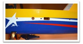
Locate the horizontal stabilizer pocket. Use an iron to seal the covering around the edges of the pocket before trimming. Use a new hobby knife blade to cut though the covering.
