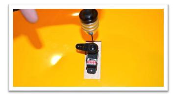
Assemble a ball link to each end of a connecting rod. Use a socket head screw, a flat washer and a nylon lock nut to connect a ball link to the servo control horn. (The brass ball in the link is offset. The larger reveal side should be against the control horn and servo arm shown below.)
