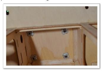
Use an "X" mount with a mounting bolt circle of 75mm to mount your motor. Use the supplied 4mm bolts and washers. Add removable thread locker during installation.
