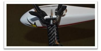
Use a machine screw and washer to draw a blind nut into the wheel pant.
