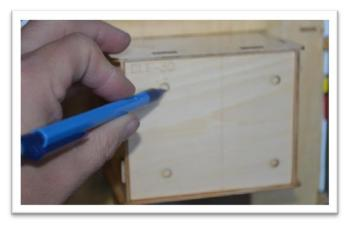
Drill 3/16" (4.5mm) holes through the firewall. Then use a 4mm bolt and washer to draw blind nuts into the back of the firewall.
