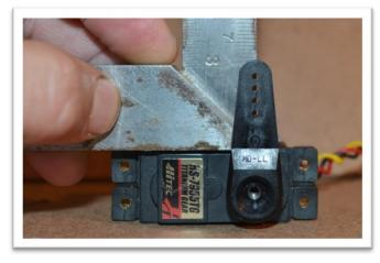
Attach the servo wire to the installation string and gently pull the wire through the wing as you insert the servo into the wing. (Depending on the length of the servo wire provided it may be necessary to install a servo extension wire before installing through the wing.)
