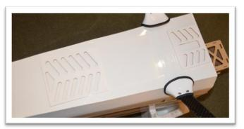
If you plan on using canister style exhaust leave the exhaust tunnel open. Install the provided pipe mounts in the tunnel and fuselage venting.
