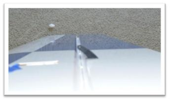
With the control horn in position apply painter's masking tape around the control horn base. Put the tape up to the base edge. Not under or over it.
