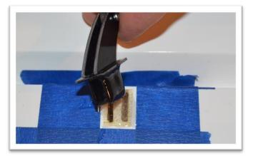
Wipe away excess epoxy using a paper towel soaked with denatured alcohol. Use an upward rolling motion as you wipe the excess epoxy to lift it from the surface. This helps reduce smearing the epoxy.
