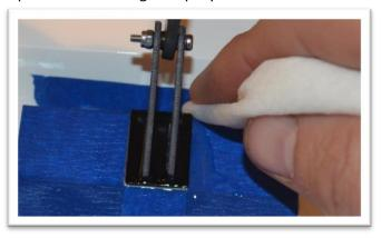
Check the alignment along the hinge line as you did when you test fit the control horn. Reposition as needed. Allow the epoxy to partially cure. Peel away the masking tape after the epoxy is securely holding the control horn in place and still soft enough to easily remove the tape. Set aside and let the epoxy fully cure. (Repeat on second elevator half if you will be using 2 elevator servos.)
