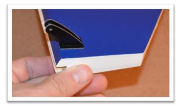
With the control horn in position apply painter's masking tape around the control horn base. Put the tape up to the base edge. Not under or over it.
