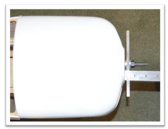
The prop backer plate will be about 6.3" (160mm) from the fuselage firewall.
