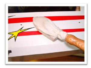
At 200-220°F (93-104°C) the adhesive on UltraCote® becomes active allowing the covering to be attached to the model. While 220° will fully bond the covering to the model it is well below the temperature that causes UltraCote® to shrink.
