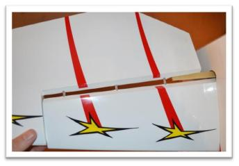
Apply petroleum jelly (Vaseline) to the center hinge pin portion of each hinge. This will help prevent glue from getting into the hinge when gluing then into the elevator. Avoid getting petroleum jelly on the barbed portion of the pin. If you do clean it off with alcohol.
