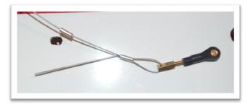
Loop around and back through the crush sleeve again.
