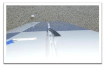
Allow the epoxy to partially cure. Peel away the masking tape after the epoxy is securely holding the control horn in place and still soft enough to easily remove the tape. Set the wing aside and let the epoxy fully cure.
