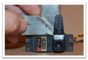
Reinstall the servo. Assemble a connecting rod and ball link and to elevator ball link. Check the length of the assembly to the servo arm with the elevator aligned with the stabilizer at the leading edge. Once the correct length of the assembly is found connect it to the servo arm using the provided machine screws washer and lock nut. (Turn on the transmitter, receiver and servo while making adjusting to the connecting rod. This will keep the servo in its correct position.)
