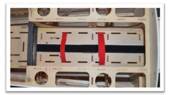
Use the balsa sheet and 2mm wood screws provided to cover the exhaust tunnel. Leaving this open may trap air and result in unwanted flight characteristics.
