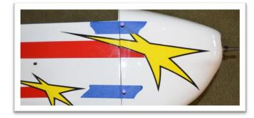
Remove the cowl and use a 3/32" drill to open up the pin holes. (Or drill at the marked locations.)
