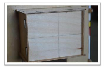
Use these centerlines to position the mounting holes for the engine you decide to use. (You can use the DLE30 template if your engine uses a 54mm X 70mm hole pattern. Some engine manufactures provide templates to help locate the mounting holes, fuel line and throttle linkage. Before using these templates measure them after printing to make sure they have printed to scale.)
