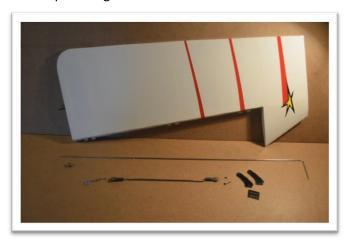
Notice that the control horns for the push-pull system shown at the top of this picture are longer then the pull-pull control horns.
