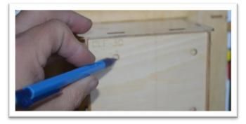
Drill the mounting holes then temporarily mount your engine standoff and the engine. (A DLE35RA is shown.)
