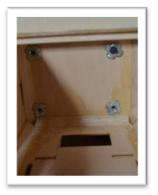
Use 4mm bolts and washers to secure the motor box to the fire wall. Apply removable thread locker to the bolts during assembly.
