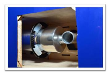
Cut the cowl as needed to clear the engine head, spark plug and muffler. Cut a large opening at the rear of the cowl to keep your engine running cool.
