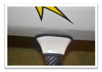
Ensure all set screws are tight on the pre-assembled tail wheel assembly.
