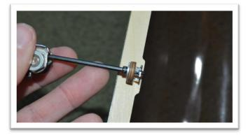
Secure the canopy to the fuselage.
