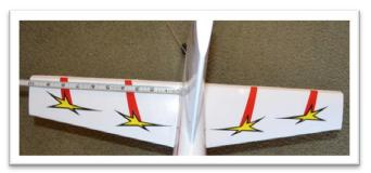
Install and center the main wing tube. Look at the plane from the back forward to make sure that the horizontal stabilizer is parallel with the wing tube. Notice that the horizontal stabilizer is tapered which may obscure the actual alignment. If the stabilizer is not aligned use shims or sand inside the pocket until it's parallel.
