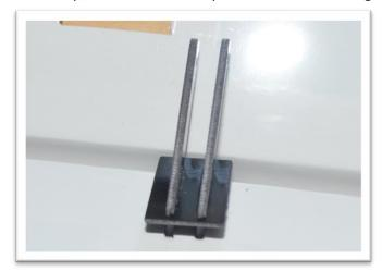
Check the alignment of the control horn to the hinge center line. The linkage hole in the control horn should be aligned with the hinge centerline.
