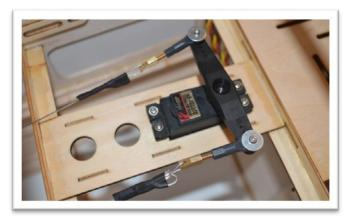
Tape the rudder in position aligned to the vertical stabilizer. With the servo powered up and centered repeat the crimping process on the rudder end of the cable. Before you crimp the crush sleeves make sure the cable is not looped around the cable eye at the servo end. Pull the cable snug. You don't need to make the cable a guitar string tight.
