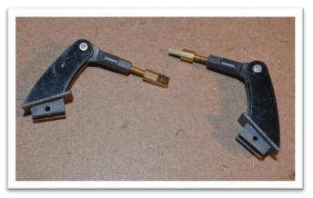
Tests fit the control horns to the slots and align with the hinge line. The control horns should be symmetrical about the hinge line.
