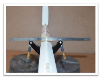
Use 30 minute epoxy to glue the control horns in place. Check the alignment, peal the masking tape away and set aside for the epoxy to cure.
