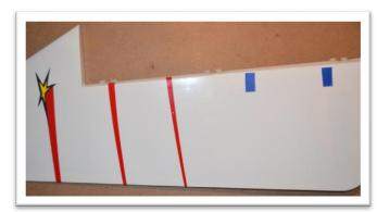
Cut the rudder covering to expose the control horn slots on both sides of the rudder as you did for the ailerons and elevator. Test fit the control horns, mask off the area surrounding the control horns and use a fresh knife blade and cut the covering as you did with the ailerons and elevator.
