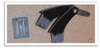
Apply epoxy to the slots in the elevator. Use a pin to help push some epoxy into the slots.
