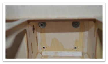
The distance between the prop backer plate and the firewall should be 6.3" (160mm). This will provide space between the spinner and the cowl.
