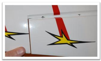
Practice assembling the elevator, hinges and jointer plate together without glue so things go smoothly when you glue it all together.
