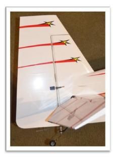
Install the rudder servo into the fuselage and pre-drill for servo mounting screws using a 1/16" drill. Install the servo with the wood screws that came with your servos. Remove the screws and servo and apply a drop of thin CA glue into each mounting screw hole. This will harden the wood around the screws and provide a more secure installation. (Allow the CA glue to dry before reinstalling the servo.)
