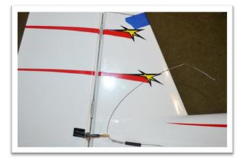
Remove the tape and adjust the cable lengths to center the rudder by turning the cable eyes into the ball links.
