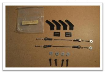
Test fit the control horn halves in the slot first individually, then as an assembly. The fit should be snug.
