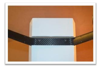
Place the wood filler block over the landing gear. Pay attention to the fit as it is directional. We suggest using a piece of white covering or clear packing tape to hold the filler block in position.
