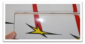
A small round file can be used to give the hinges some clearance. Cleaning out the holes will also help you close up any gap. Turn a 1/8" drill into the holes by hand.
