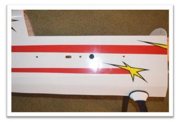
Carefully locate the horizontal stabilizer pocket. Use a trim iron to seal the covering around the edges of the pocket before trimming. Use a new hobby knife blade to cut though the covering.
