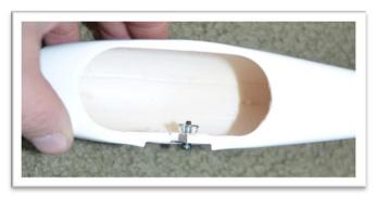
Slide the wheel onto the axel. Add the wheel collar and tighten the set screw. Ensure it rotates freely. Put the wheel and axel into the wheel pant then put the axel threads through the landing gear.
