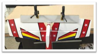
Carefully remove "masking" tape before the epoxy fully sets. But do not remove the tape at the stabilizer and elevator counter balance until epoxy is fully cured.
