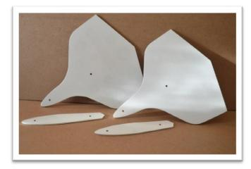
The wing tips have a blind nut installed beneath the covering. Use a hobby knife to trim away the covering. (Use the holes in a spacer plate to help locate the holes in the wing tip.) Assemble the spacer plate and the side force generator to the wing with the supplied screws and washers.
