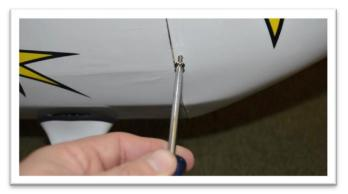
Apply thin CA glue to the mounting tabs and screw holes. (Allow plenty of time for the CA glue to dry before reinstalling the cowl.)
