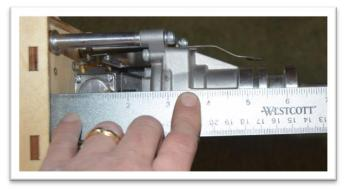
Check for clearance between the firewall and the carburetor. This distance should be noted in your engine's manual. If you don't have at least the recommended space cut an opening in the firewall so the carburetor can get air.
