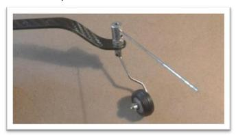
Use the landing gear fasteners locate on the bottom of the fuselage along with 2 flat washers located in the landing gear package to mount the carbon fiber landing gear. Add a drop to removable thread locker to screws during assembly.
