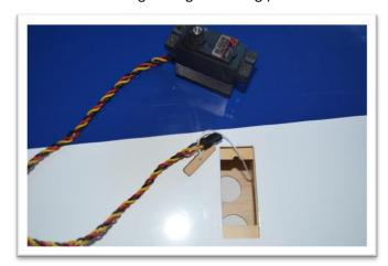
Secure wire extensions to servo leads using shrink wrap or a safety clip.
