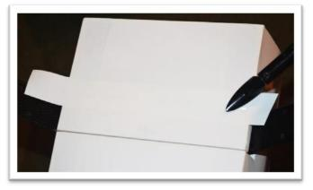
Install the landing gear cuffs with the holes towards the bottom of the airplane. Use a flat blade screw driver with a gentle twist to help slide the cuff over the landing gear.
