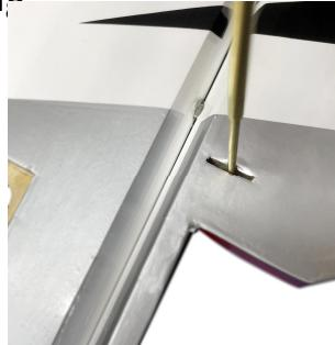
2. Use sand paper to scuff the root of control horns for a good glue bond. Try to insert it into the mounting slots to adjust the position first.
