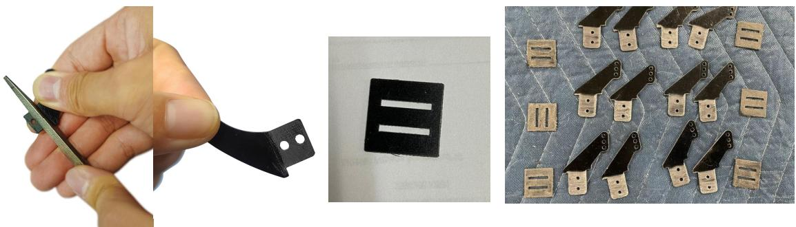
3. Put the control horns reinforcing piece, drop the horns in the holes, positioned correctly when the horns are directly above the hinge line, then stick masking tape around the reinforcing piece as shown in the picture, cut about 1mm inside with a knife and remove the covering, below to expose the pre-cut slots.
